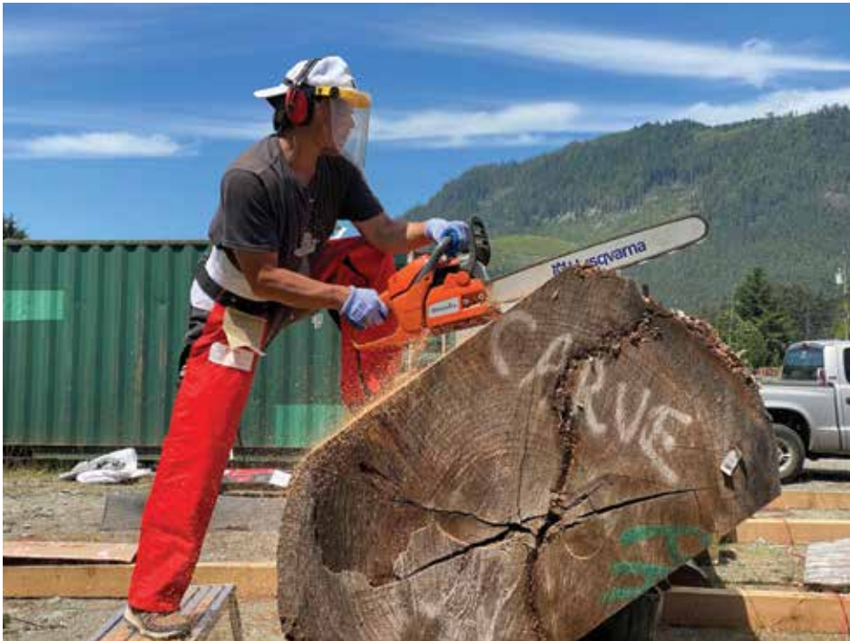
Makah master carver Micah McCarty roughs out the canoe shape with a chainsaw. PHOTO: SOPHIE ADAMS
