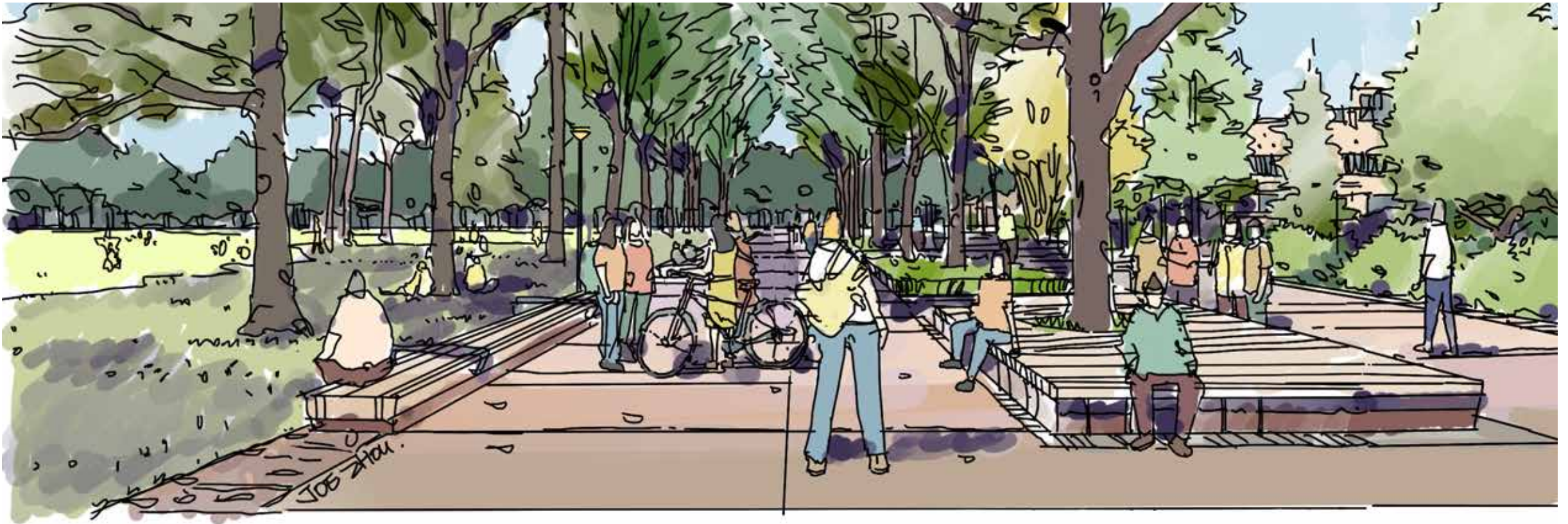
Figure 1.2.1 Central Campus Greenway with widened pathway, and seating and edge plantings to protect tree root zones
