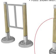
Notched post for single pole mounting. Sign will mount through back of post. Holes to be drilled and tapped through structural sign frame to accept stainless steel machine bolts. Matching holes to be drilled in back of post and finished with wooden plugs after installation.
