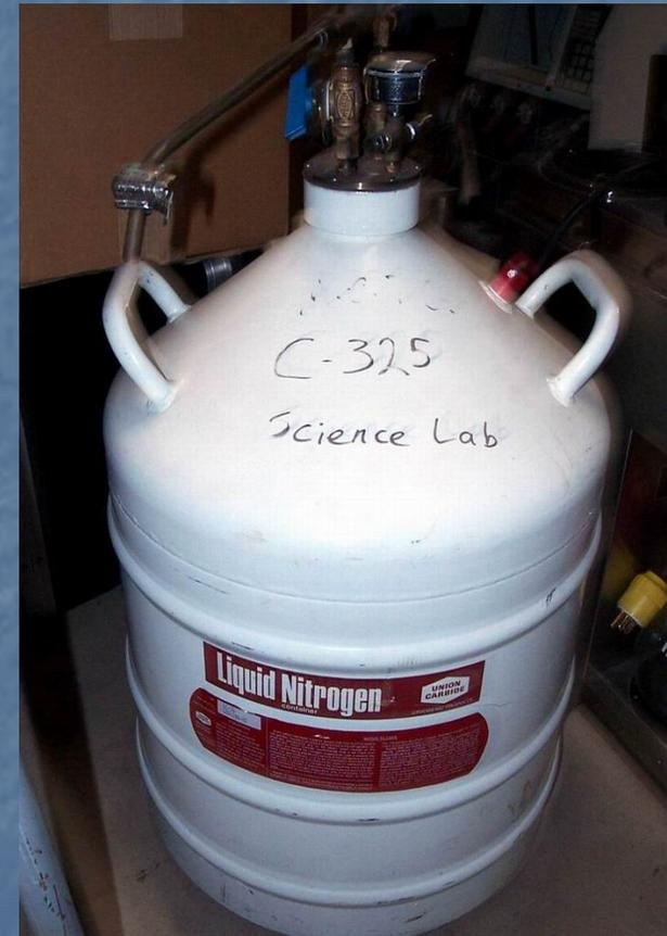
Use only containers specially designed to hold liquid nitrogen
