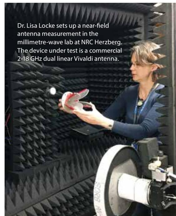
Dr. Lisa Locke sets up a near-field antenna measurement in the millimetre-wave lab at NRC Herzberg. The device under test is a commercial 2-18 GHz dual linear Vivaldi antenna.
