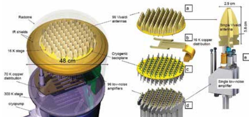
Left panel: A phased array feed receiver. A cryopump cools the 96 copper antennas and low noise amplifiers from room temperature to 16 K. A dewar and composite radome maintain an extremely high vacuum. Incoming radiant heat is reduced through the radome with many layers of infrared shielding and concentric metal shields. *Image courtesy of R. Wierzbicki.*
