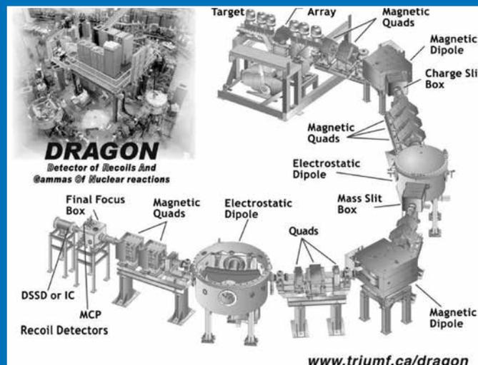
Located in the ISAC facility at TRIUMF in Vancouver, British Columbia, DRAGON is an apparatus designed to measure the rates of nuclear reactions important in astrophysics. Of particular interest are the reactions that made the elements around us; the nucleosynthesis reactions, which occur in the explosive environments of novae, supernovae and x-ray bursters.
