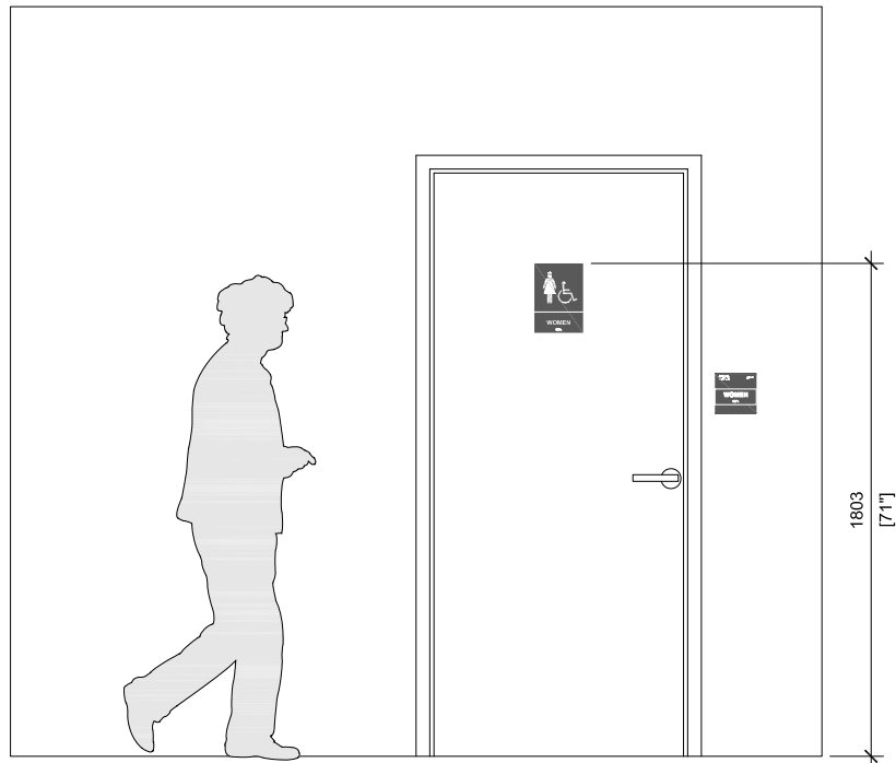
Installation of Washroom Door Signs
