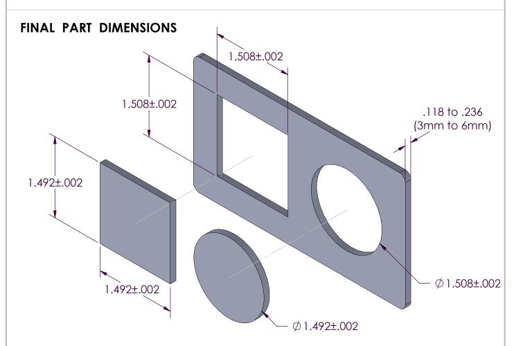
WIDTH OF CUT (KERF) IS 0.008", SO FEMALE CAVITIES ARE 0.008" LARGER THAN DRAFTED, AND MALE COUNTERPARTS ARE 0.008" SMALLER THAN DRAFTED (0.004" ON EACH SIDE)
