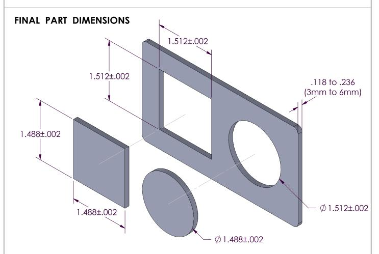
WIDTH OF CUT (KERF) IS 0.012", SO FEMALE CAVITIES ARE 0.012" LARGER THAN DRAFTED, AND MALE COUNTERPARTS ARE 0.010" SMALLER THAN DRAFTED (0.006" ON EACH SIDE)
